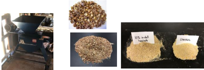
In-shell hazelnuts were pulverized to 1772 \mu m using a roller mill prior to mixing with control diet
