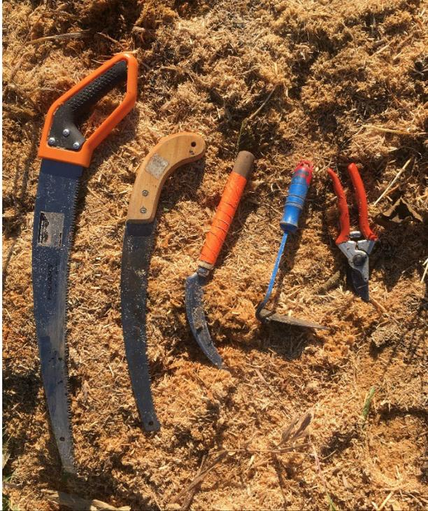
**Tools for harvesting layers. From left to right: two types of pruning saws and a rice knife (also called a Japanese sickle) for cutting masses of stems together; a hand hoe for digging into soil beneath a root if needed, and pruning shears for cutting off individual stems.**
