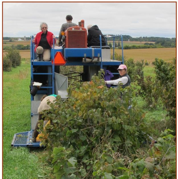
**Photo 1.** In-husk nut clusters are harvested directly from the hedgerows. Growers are currently using blueberry harvesters, but work is underway to develop more effective equipment. Photo: Dave Bohnhoff
