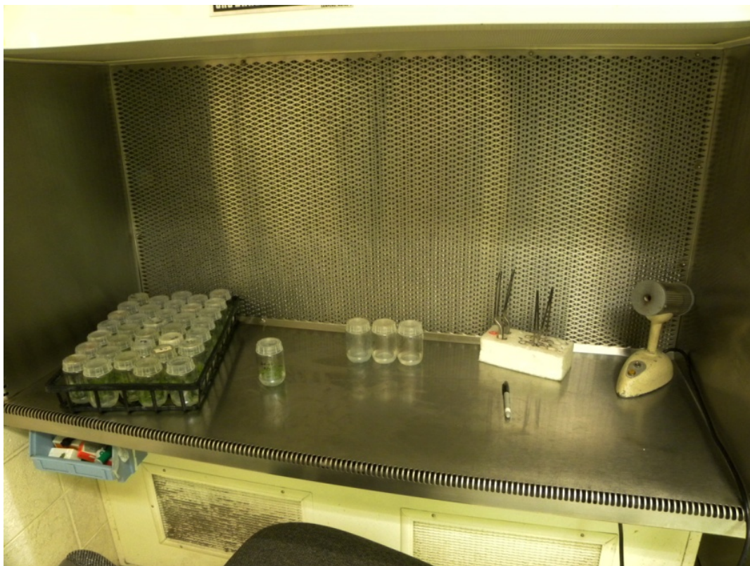
Fig. 3. A sterile transfer cabinet used to perform sterile transfers. Stems from hazelnut cultures (left in picture) will be cut and placed on new media (center) using surgical steel quality sterilized tools (right).
