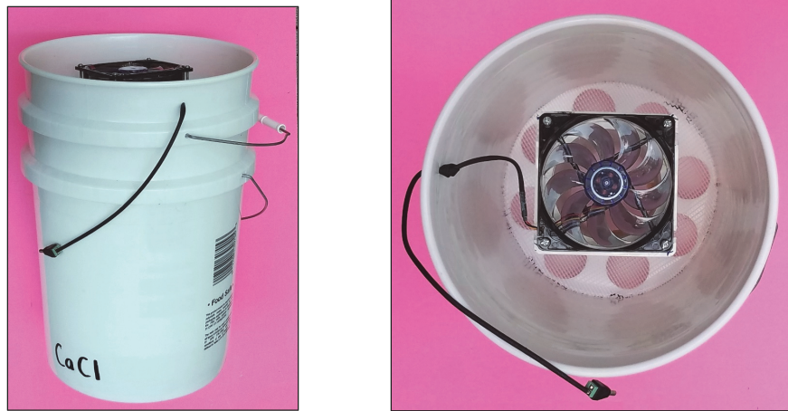
Figure 3. Side and top views of a biomaterial moisture conditioning unit (shown without snap-on cover).
