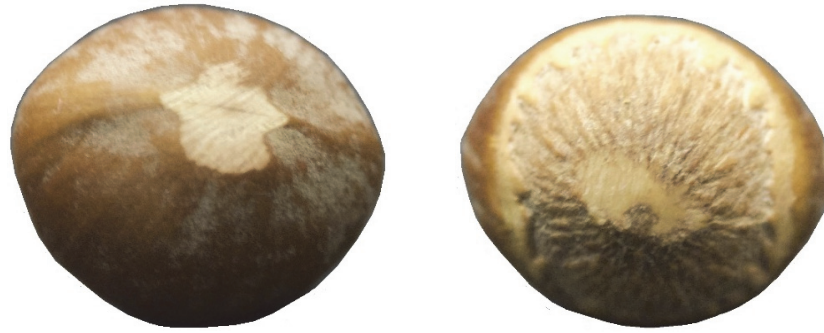
Figure 3. Nuts sanded for compression along the X-axis.
