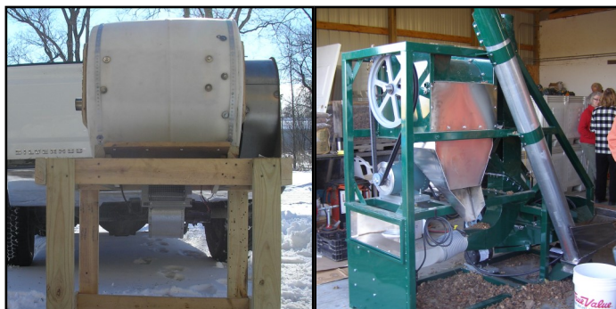
Photo 22 Low-cost barrel husker to remove husks from in-shell nuts (left). The X2000 husker is based on the barrel husker, but can be continuously fed (right).
