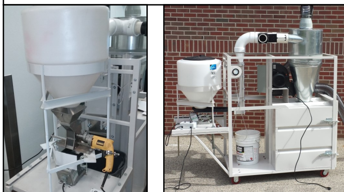
Photo 24 (left). Drill Cracker being fed with from a plastic hopper. Photo 25 (right). Badger aspirator to separate shell fragments from kernels after cracking.
