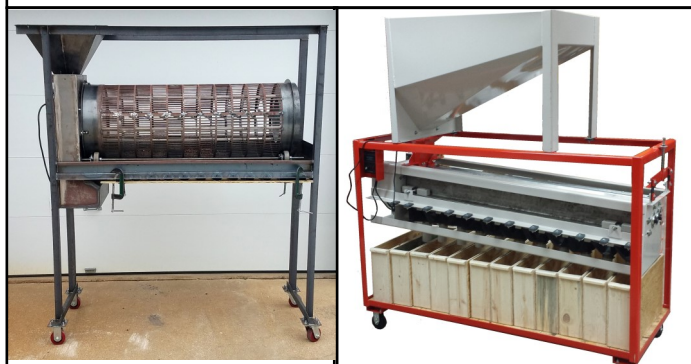
Photo 23. Student designed rotary-drum sizer (left) and the Badger roller-sizer (right) separate in-shell nuts into different size classes.
