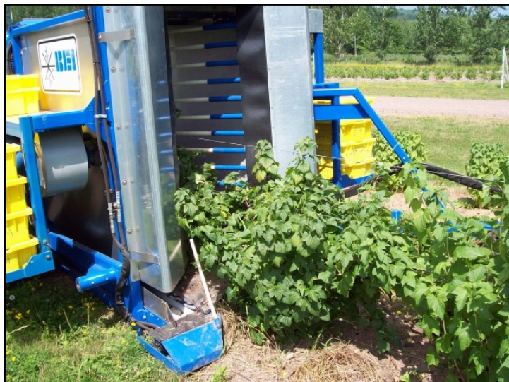
Photo 20. BEI harvester showing the sway bars used to detach the fruit or nuts from the plant as they pass through the harvester tunnel. The unit shown here is designed for high-bush blueberries before they reach mature size. It is being used here for black currants.
