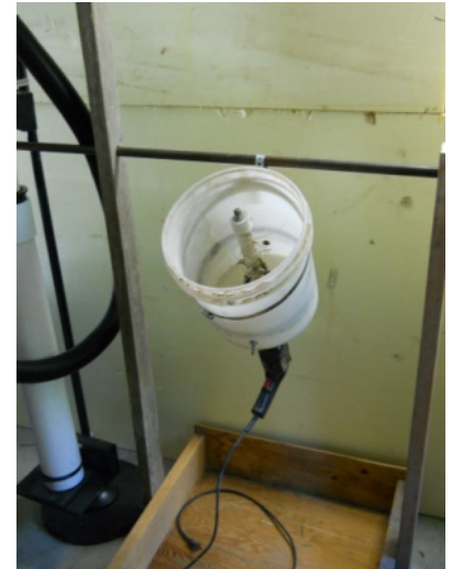
A corded drill provides the power for this batch-type husker. The bucket hangs freely keeping the angle at roughly 45 degrees.
