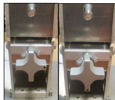
Photo 1. Narrowing the gap between the spindle and anvil on the Drill Cracker® is done by turning the knob clockwise. For methods evaluated in this study, the knob was turned 1/4 turn between passes as illustrated by the black dots on the knob in the photos above.
