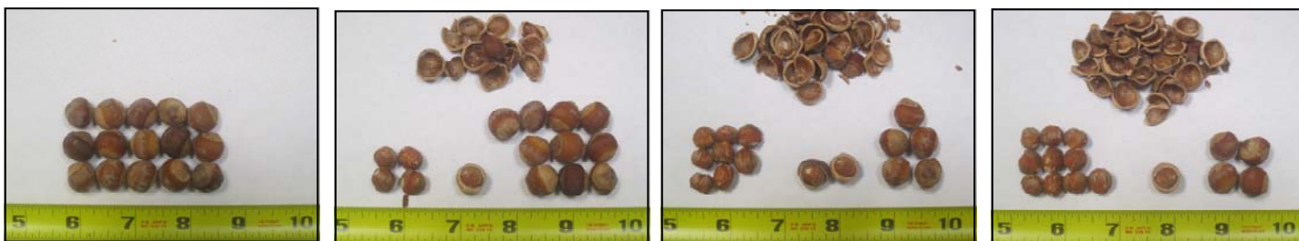
Photos 2-5. Photo 2 shows a typical starting sample of 15 nuts. Photos 3-5 show the increase in whole kernels produced with each successive pass through the cracker.
