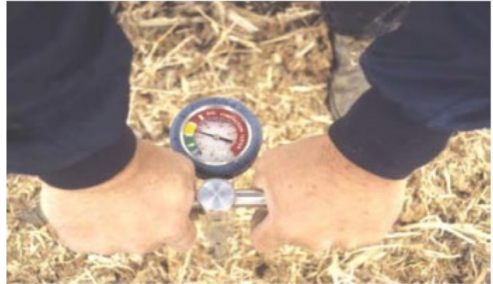
A soil penetrometer is one tool to check soil compaction depth. Source: NRCS Grigar Midland County
