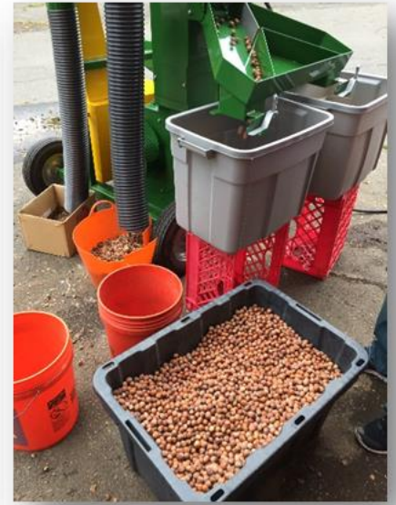
The Italian-made Chianchia 2-stage cleaning machine removes sticks, stones, shells, etc. and even blank nuts.
