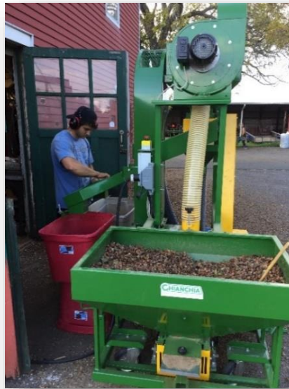
The Italian-made Chianchia 2-stage cleaning machine removes sticks, stones, shells, etc. and even blank nuts.
