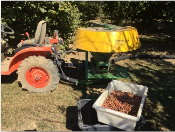
Harvester powered by Kubota narrow nursery tractor to fit down tight rows.
