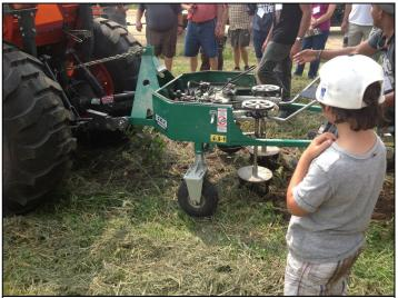
**Photo 6.** Specialized equipment for cultivating in shrub and tree plantings should be considered for larger-scale plantings. Equipment such as the Eco-Weeder<sup>™</sup> shown here or the weed badger allow the operator to cultivate weeds between the plants.
