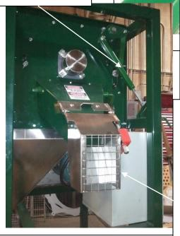
Safety shielding inside cylinder drive door and on nut discharge outlet
